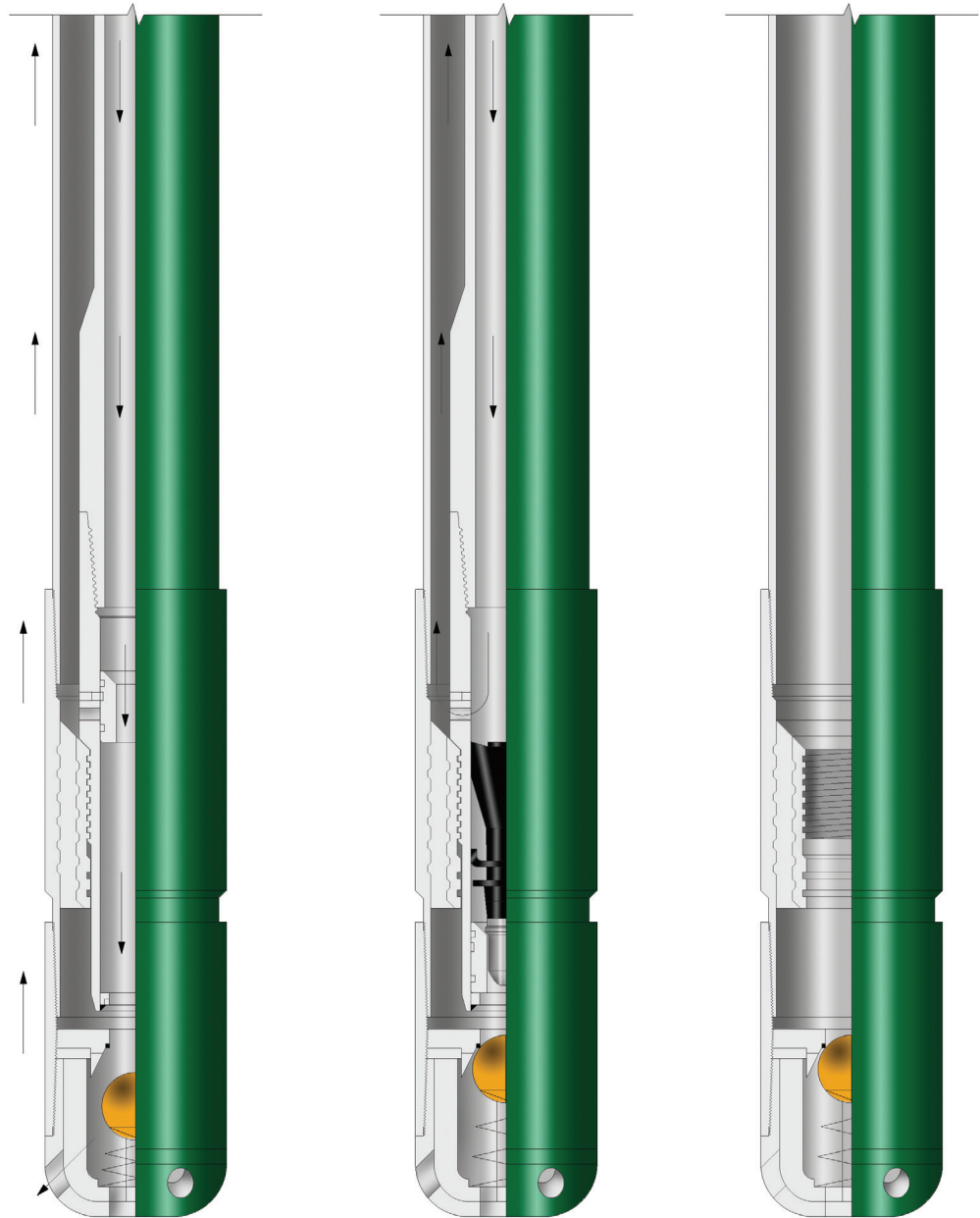
SETTING TOOL THREADED INTO CEMENTING SHOE ASSEMBLY. CIRCULATING/CEMENTING ON BOTTOM.
